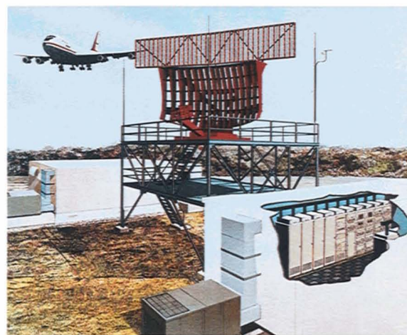
Fig. 17—Mode-S engineering-model sensor.
