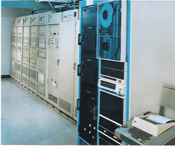
Fig. 18—ARIES with the Mode-S engineering-model sensor.
